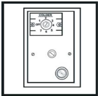
Find the screw type with the numbers around it. This switch enables the fluctuation of the size ice size.
